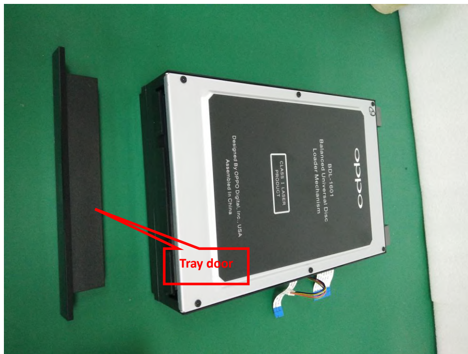
3.3.3 The loader component and the tray door that taken out
