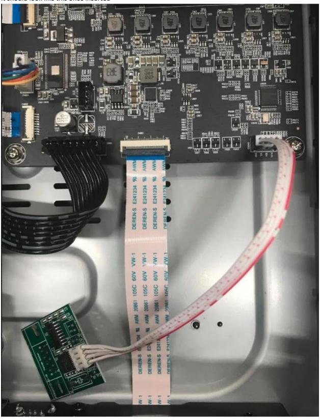
5) Use the provided Plastic tie to secure the upgrade board to the player around the cables to prevent it from moving around.
