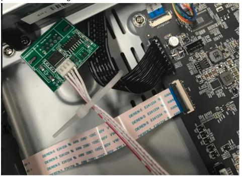
6) Tighten the Tie to secure the board
