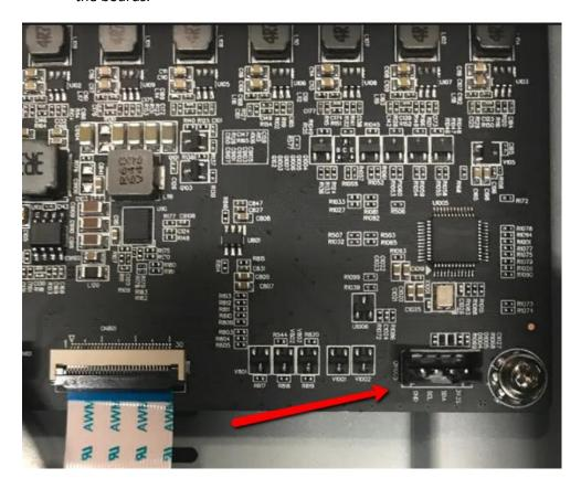
3) Insert the white cable from the upgrade board into the connector
